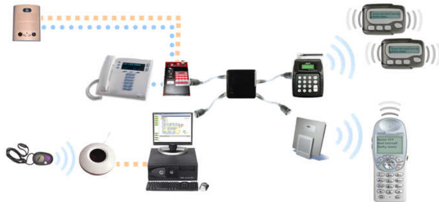
After: Added an EZInc™ Pro-TAP module to connect a wireless system & a wireless phone system output The existing nurse call only needed the new phone extensions programmed into it; all assignments remain on the nurse call.
