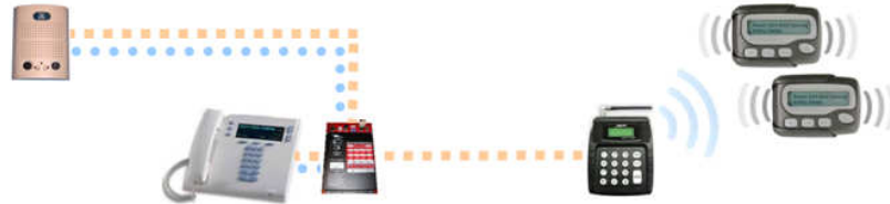
Before: Existing system with a nurse call system tied into pocket paging via a TAP serial connection
